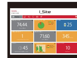
Visualizes a wide range of data such as vehicle operations by each operator, detected shocks and battery usage.
